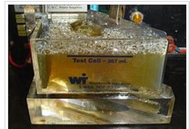
A zinc solution tested in a hull cell
