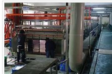
Copper electroplating machine for layering PCBs
