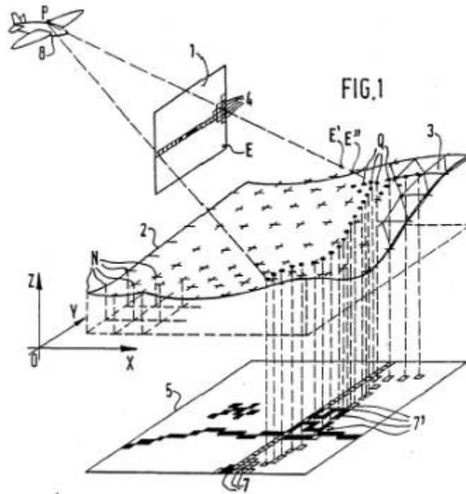
Mouchot interpolates elevation points from a digital elevation database, maps them onto a color picture, and displays the points in perspective. The big question is how he does the perspective.
