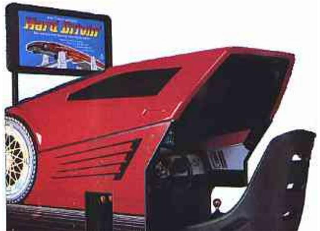
The force feedback was controlled by the Car Model, which mathematically describes the physics of how the parts of the car (engine, transmission, springs, shock absorbers, tires, etc.) react to each other, to the road, and to the driver's inputs.
