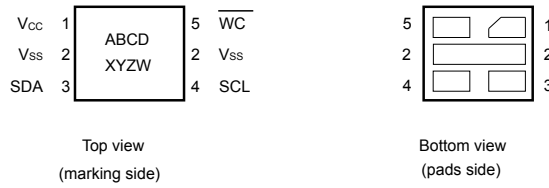
Figure 3. UDFPN5 (DFN5) package connections
