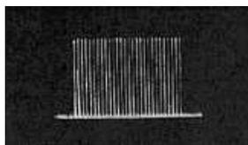
*A Spectrum Analyzer Photo of a Frequency Hop (FH) Spread Spectrum signal.*
