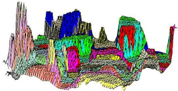
After you have used the digital elevation points to produce polygons you can shade and blend the polygons so that the underlying polygons may no longer be obvious. Honeywell did an excellent job in their IPFD (Instrument Primary Flight Display) [\[Ref. 9\]](#):
