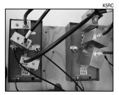
Figure 3 — Amplifier RF input switching: SixPaks with band-pass filters for each band
