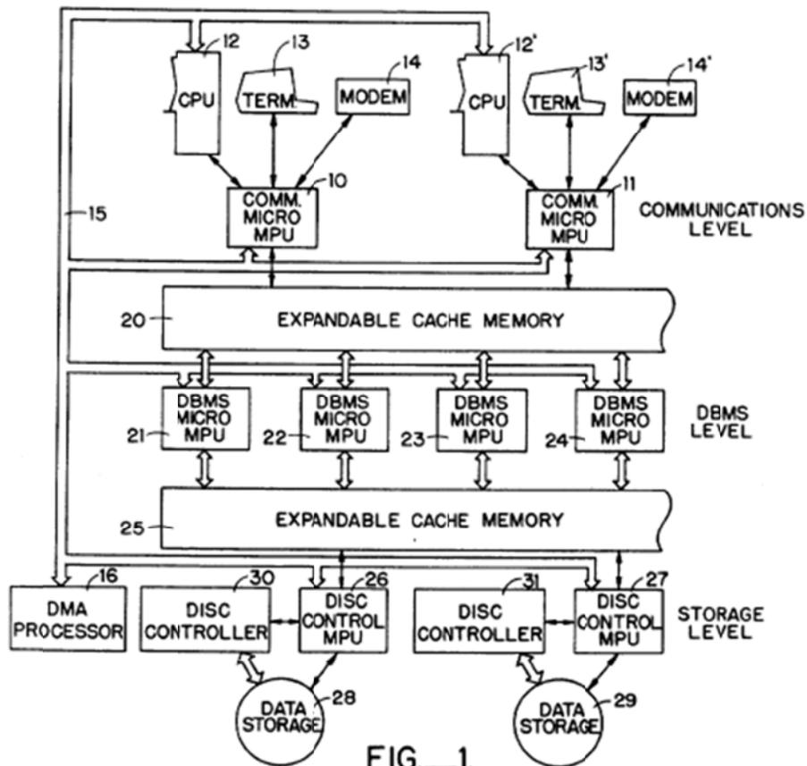
Millard's Fig. 1 discloses an information storage facility with multiple level processors wherein a direct memory access bus is provided which enables high speed data transfer among the several processors included within the storage facility and also external host computers or intelligent terminals (Abstract).
