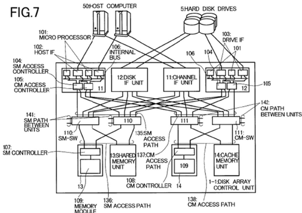
Fujimoto's Fig. 7 discloses a channel IF unit 11 that includes two microprocessors 101 for controlling the data transaction with the host computers 50, an SM access controller 104 for controlling the access to the shared memory units 13, and a CM access controller 105 for controlling the access to the cache memory units 14 (col. 7, ll. 6-15).
