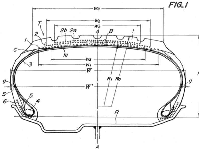
Figure 1 depicts a sectional view of a tire with a carcass 3, and a composite belt B. Belt B includes two layers:
