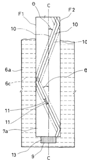
Figure 2 depicts the zig-zag pattern of the wound tape 10 forming the breaker 7. Ueyoko teaches that the zig-zag pattern improves durability by avoiding breaker edge loosening. (Ueyoko, col. 3, ll. 26-27.)
